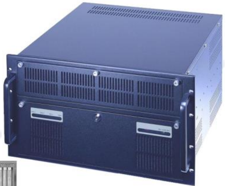
Replaceable rear panel to support Backplane and ATX motherboard
