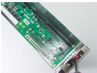
Place the backplane bracket with CPU card inside back to the chassis, and secure with four screws  Insert the CPU Card to the backplane socket and secure with original screw from I/O slot bracket
