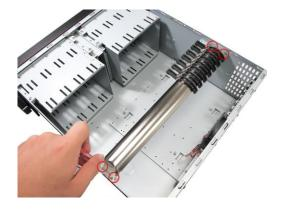
Correctly position the PSU at the rear of the chassis with the power switch and cable socket both facing outwards. Secure the PSU by inserting four retention screws through the rear of the chassis
