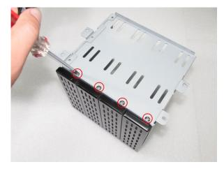
Carefully insert the ODD drive into the drive tray, and secure the drive by inserting eight retention screws (four on each side) through the sides of the drive tray
