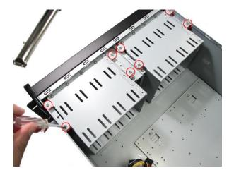
Remove the screws (2 screws for one cover) to remove the drive cage covers.
