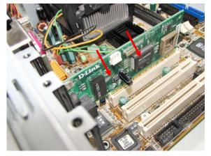
1. Slide the Expansion card into the socket 2. Secure the expansion card I/O bracket with screw
