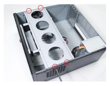
Lay the motherboard to the chassis and secure to the standoff below with the screws provided by the board manufacturer
