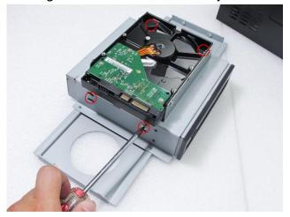
6. For additional 3.5" drive, carefully place the drive to the inner right side of the chassis, and secure the drive with four retention screws
