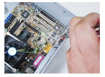
2. Insert the Expansion card into the motherboard slot and card by the previously removed slot cover screw
