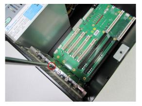
Slide the Expansion card into the socket on the backplane reserved for the Expansion card. 3. Secure the expansion card I/O bracket with screw
