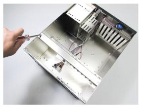
Correctly position the PSU at the rear of the chassis with the power switch and cable socket both facing outwards. Secure the PSU by inserting four retention screws through the rear of the chassis
