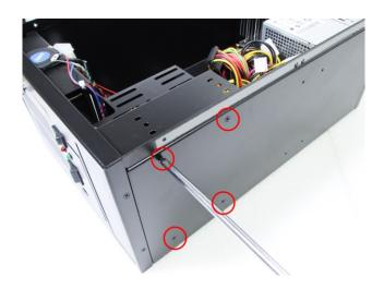
Remove the screws to remove the drive cage covers. Secure the Optical drive and/or hard disk drive to the cage.
