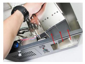
Remove the screws (2 screws for one cover) to remove the drive cage covers. Secure the Optical drive and/or hard disk drive to the cage.
