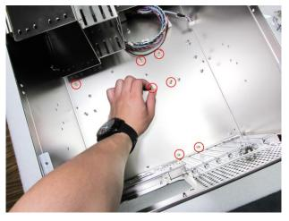
Lay the motherboard to chassis and secured with screws to the standoff below
