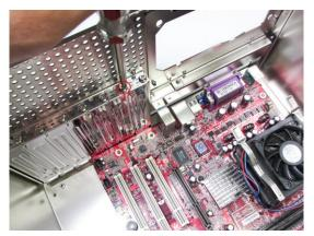
2. Slide the Expansion card into the socket on the motherboard reserved for the Expansion card. 3. Secure the expansion card I/O bracket with screw
