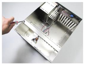
Correctly position the PSU at the rear of the chassis with the power switch and cable socket both facing outwards.
