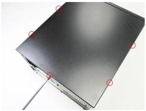
2. Slide the cover toward rear of the chassis, then lift the cover off the chassis
